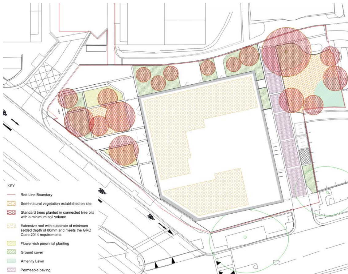
Image 47 (above): Site layout, illustrating in red, the arrangement of the 16 trees proposed.
